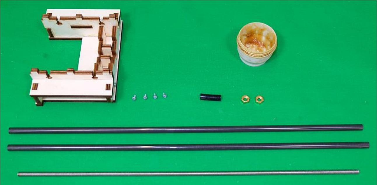
As with the threaded rods of the gantry, screw in the nuts on the side marked in blue or green and screw the sleeve on the opposite side 10mm. Lubricate the threaded rod, spread the grease with the nuts and remove the excess.
