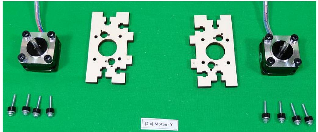
Center the plywood piece on the engine slowly. Roman numerals should be visible and the axis must protrude from the center of the circle. Attention! The engines are slightly skewed to the edge parts of the plywood.
