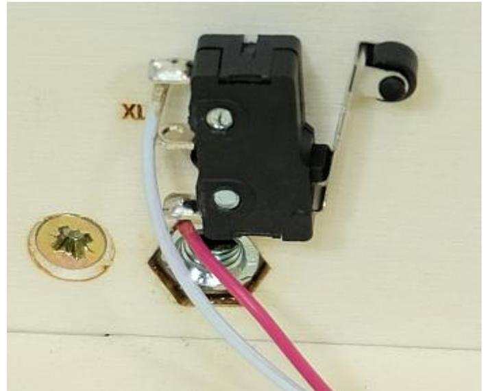
For **XC and XL**, place the screws in the left position of the setting area and tighten moderately, without marking the wood so as to be able to adjust the position later.
