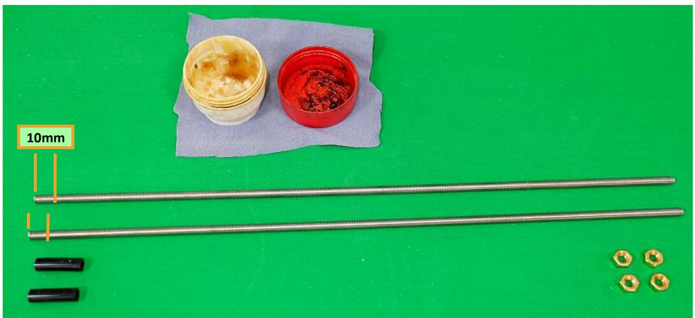
Grease the threaded rods and make the nuts circulate from one end to another in order to spread the grease. Wipe away the excess grease. You just need the nuts to turn smoothly. The grease will continue to be distributed over the entire length of the rods during the initial use of the MiniCut2d. You can use an electric screwdriver to accelerate this process.
