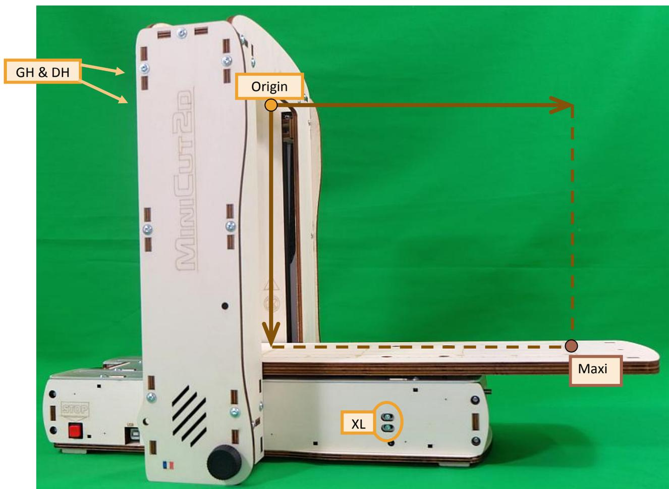
XC, GB and DB Switches determine the maximum (Maxi) movement of the plate and wire. They help maintain the mechanics of MiniCut2d for exceeding displacement during manual control.
