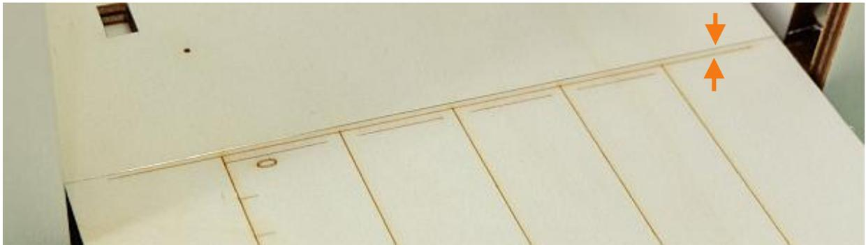
View the wire from above the MiniCut2d. The correct position is when the wire is (about) on the baseline. In the example below, it was about 1mm offset. If the wire is through, you can drag it to the springs, or rotate the springs, or realign the board.
