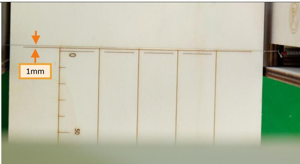
Move the plate back slightly by turning the threaded rod by hand (by the end of the rod, who exceed under the plate).
